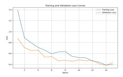
Figure 19: Validation and Training curves for AlexNet
