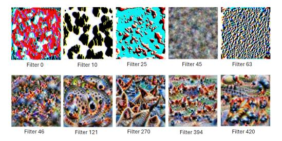
Figure 27: Feature Visualization of the first and last convolutional layer of **pre-trained VGG16**, for the binary classification task. The first layer contains 63 filters, and the last layer (index 28) has 512 filters. The top-5 filters with the highest activation values have been chosen for presentation, calculated as explained in Section 5.4.1. The first row corresponds to the first layer, and the second corresponds to the last layer.
