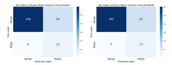
Figure 21: AlexNet vs. Resnet50: Confusion matrix on the test set for binary classification. Two confusion matrices are displayed in the image, one for each model, based on prediction results on the test set. The results show that both models can predict benign and malign samples with high accuracy, achieving a prediction rate of 82% for AlexNet and 83% for ResNet50.
