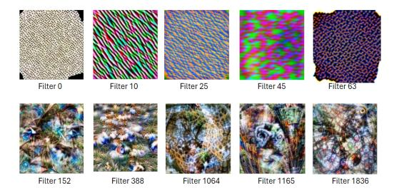
Figure 45: Feature Visualization of ResNet50 pre-trained model, binary classification. The first row represents the first layer, and the second row the last layer.
