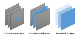
Figure 14: Different units of neural network
