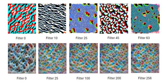
Figure 47: Feature Visualization AlexNet fine-tuned model, binary classification, malign class. The first row represents the first layer, and the second row the last layer.
