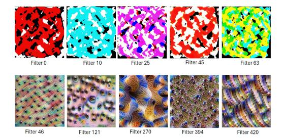
Figure 28: Feature Visualization of the first and last convolutional layer of **fine-tuned VGG16**, for the binary classification task. As with the pre-trained VGG16, the fine-tuned model uses the same filters for each layer. The first row corresponds to the first layer, and the second corresponds to the last layer.
