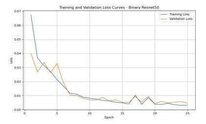
Figure 39: ResNet50 Binary classification: Convergence of Training and Validation Loss over epochs. The training loss decreases sharply and then levels off, while the validation loss decreases and then shows some fluctuation, indicating possible instability in learning as the model may be learning noise from the training data or the hyperparameters need adjustments.
