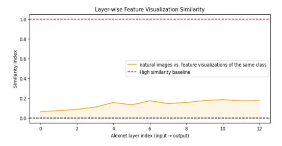
Figure 33: Empirical sanity check for **AlexNet** applied for the **binary classification** tasks. The similarity of a layer's activations caused by natural images and feature visualizations across layers (only the features block) is measured. Similarity increases in the last layers of AlexNet, because of roughly similar patterns with natural images.
