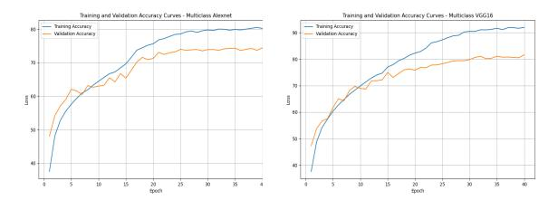
Figure 22: Accuracy curves for AlexNet (left) and VGG16 (right), multiclass classification.
