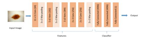
Figure 12: Alexnet Architecture
