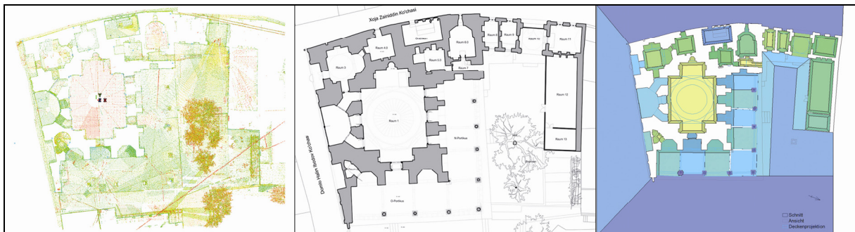
Fig. 4: The three-dimensional model generated by the laser scanner, the AutoCAD drawing, and the DMA map of the Khoja Zainuddin Mosque.
