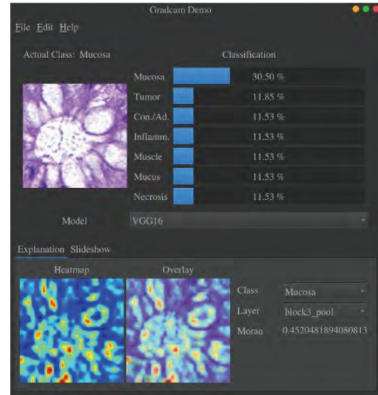
Figure 4: Interactive user interface with a view displaying the original HE image, prediction confidences produced by a CNN (which can be selected by the user) and a view for visual explanations in the form of a output heatmap, its overlay on the original image and a slideshow iterating through the heatmaps visualizations of all layers. The user can select the class for which the interface displays data as well as a specific layer for further inspection.
