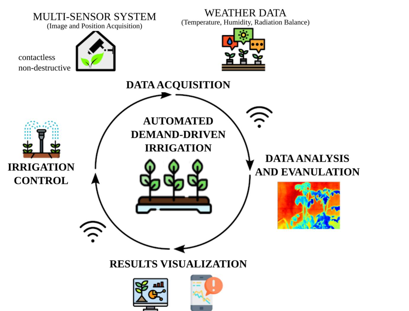
To irrigate crops according to their current water needs, continuous monitoring of the plant conditions is essential. As part of the PLANTSENS project, a multi-sensor control system was developed for automated water status measurement by combining thermal and spectral imaging within near-infrared and short-wave infrared spectrum.
