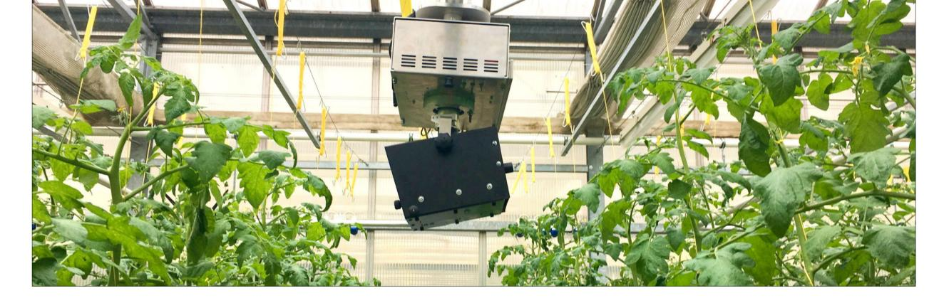
A stepper motor moves the camera system between the plant rows. The position is calculated by combining data from the IMU and the stepper motor. Additionally, the route is marked with NFC markers at both the start and end position, where the drive direction and acquisition angle change accordingly. The robot is controlled remotely by a dedicated software that uses real-time data from the sensors to mirror the status of the rover and the plants as closely as possible.
