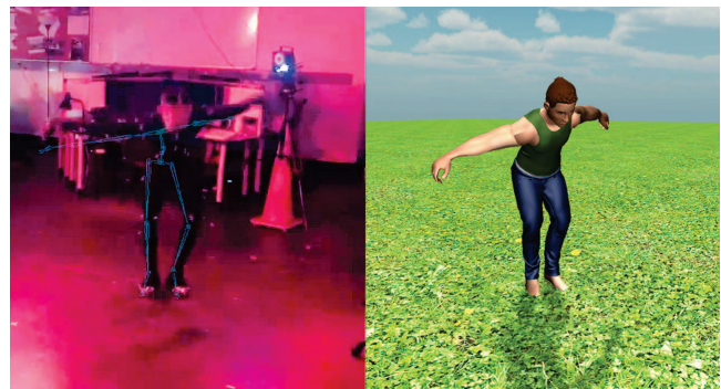
Figure 7: (Left) A trained dancer in a motion capture suit performing a hip-hop move, with the animation skeleton overlaid. (Right) The captured animation applied to a virtual character in VEnvI.
