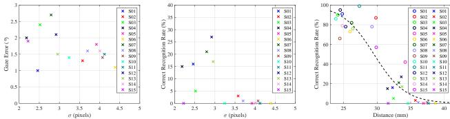
Fig. 4: Results for security and utility show that CRR is degraded by defocus ( $\sigma$ ) and increased camera distance. Circles indicate data from the in-focus configuration, while crosses indicate data from the out-of-focus configuration. The dashed line represents a sigmoid curve fit to CRR as a function of distance. Angular error measured between targets and gaze data for the out-of-focus configuration was at most  $2.7^{\circ}$ .
