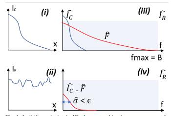
Fig. 1: In (i-ii) we depict, in 1D, the eye tracking image component  $I_C$  and the iris texture component  $I_R$ . In (iii) we show these again in the frequency domain, where the filter F is depicted as Gaussian blur and  $\hat{I}_R$  is some distribution spanning the shaded region. In (iv) we see  $I_C$  remains usable for eye tracking when the standard deviation  $\hat{\sigma}$  from  $\hat{I}_C \cdot \hat{F}$  is not less than a minimum detectable bound  $\varepsilon$ .
