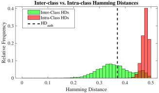
Fig. 5: A histogram of inter-class and intra-class Hamming Distances is used to determine a threshold for iris authentication.
