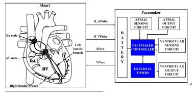
$^a{\rm Z}{\rm hao}$  and Roop, "Model Driven Design of Cardiac Pacemakers using IEC61499, CRC Press, 2015".
