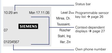
The left area contains the status bar on the first line and is followed by a five-line field for comprehensive context-specific displays. The right area is used for labeling the programmable sensor keys.
